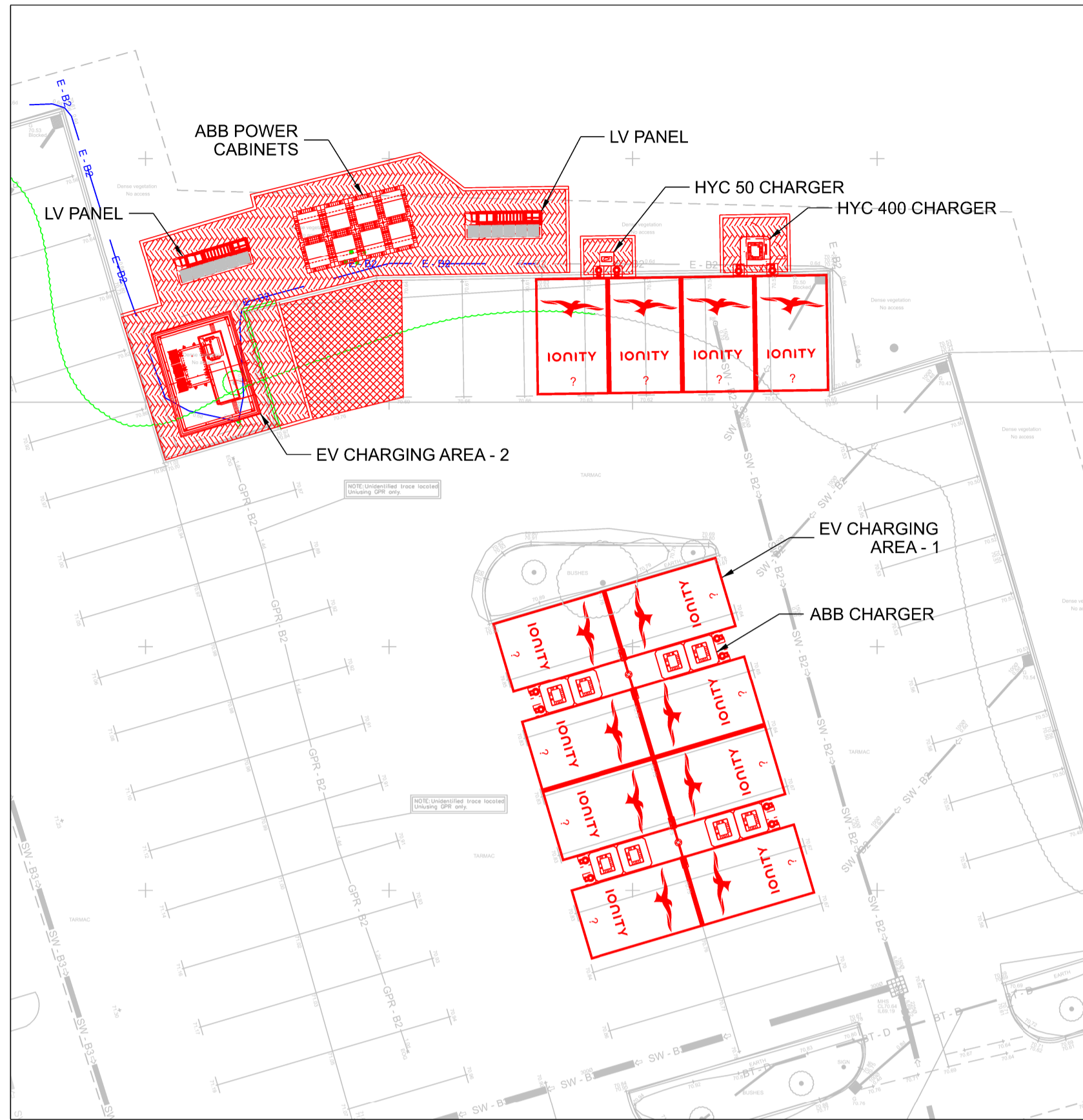
EV BAYS AND EQUIPMENT AREA PLAN SCALE 1:200
