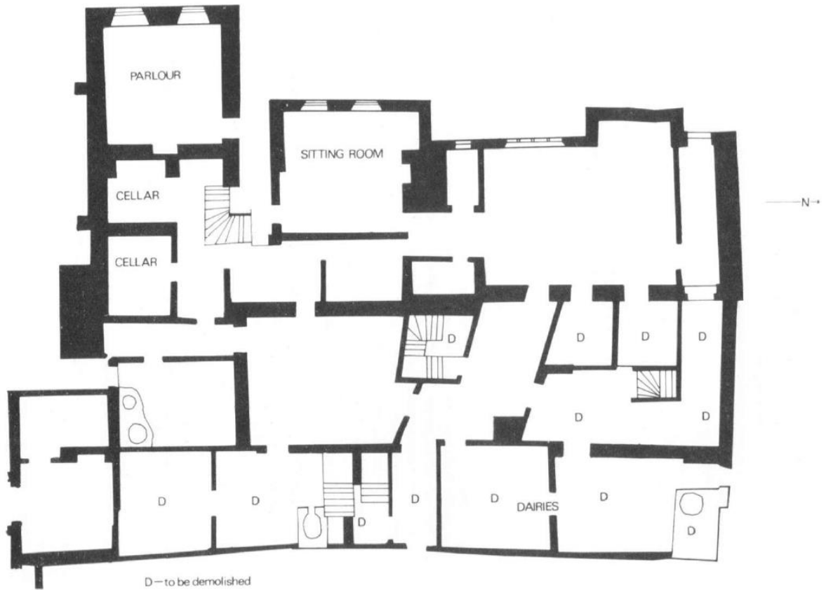
Figure 5: The Above Plan is based on documents from the 1820's, this was in preparation to carry out a phase of Demolition (see areas marked D, above) and rebuilding which would occur in 1821. This Plan was reproduced from archived material, made by The South Staffordshire Archaeological and Historical Society (1986).
