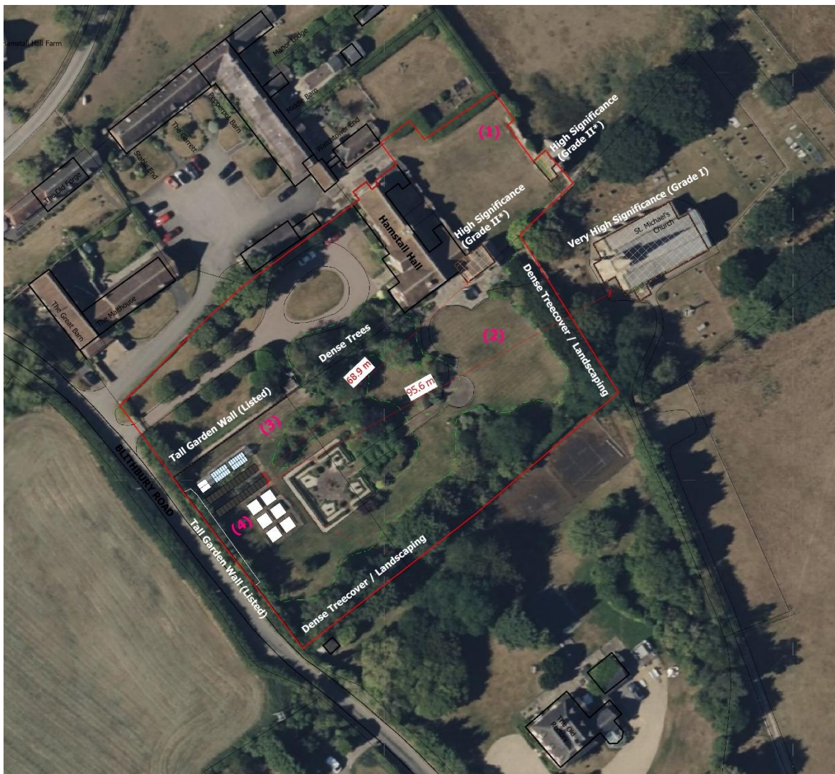
Figure 31: Strategic Options Plan - The following potential locations for 28 No. of Ground Mounted PV's were identified and assessed.
