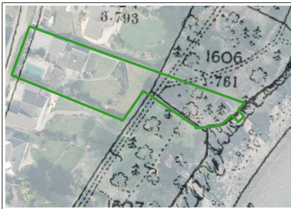
Figure 03: Historic rates of coastal erosion, Ordnance Survey dataset from 1880 overlaid onto mc satellite imagery (property outline in green).
