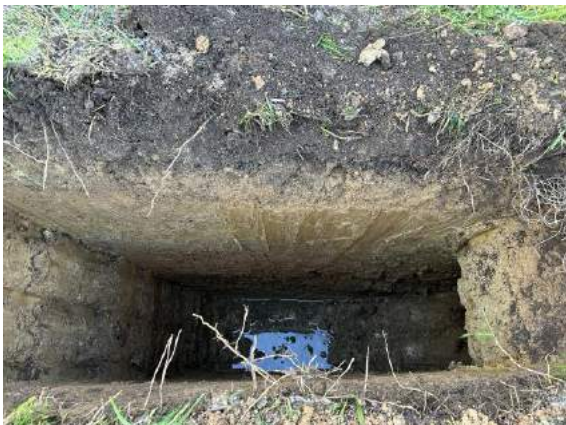
Photo 11: TP01 from Face A showing 0.10m of standing water after >20mins
