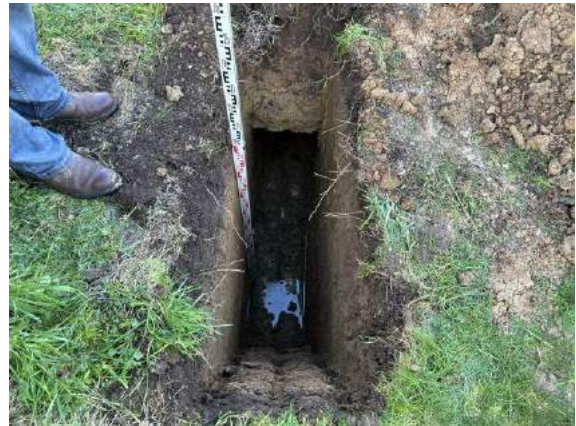
Photo 10: TP01 from Face B showing 0.10m of standing water after >20mins
