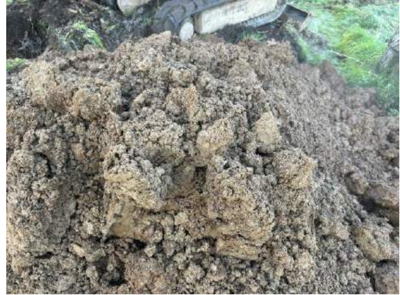
Photo 8: Spoil of TP01 (1.60 – 1.80m) looking 010 N
