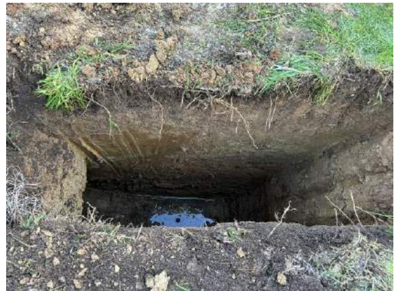
Photo 12: TP01 from Face C showing 0.10m of standing water after >20mins
