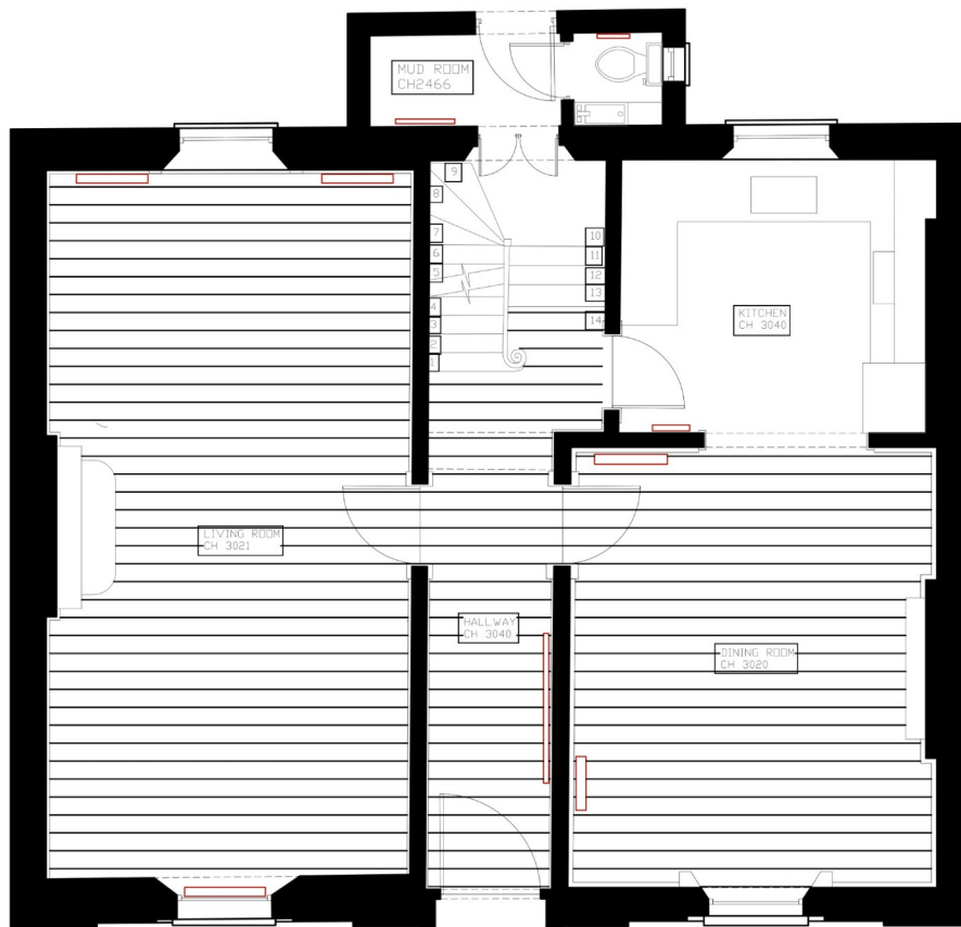
30 Hyde Vale, Greenwich Extent of original flooring restoration
