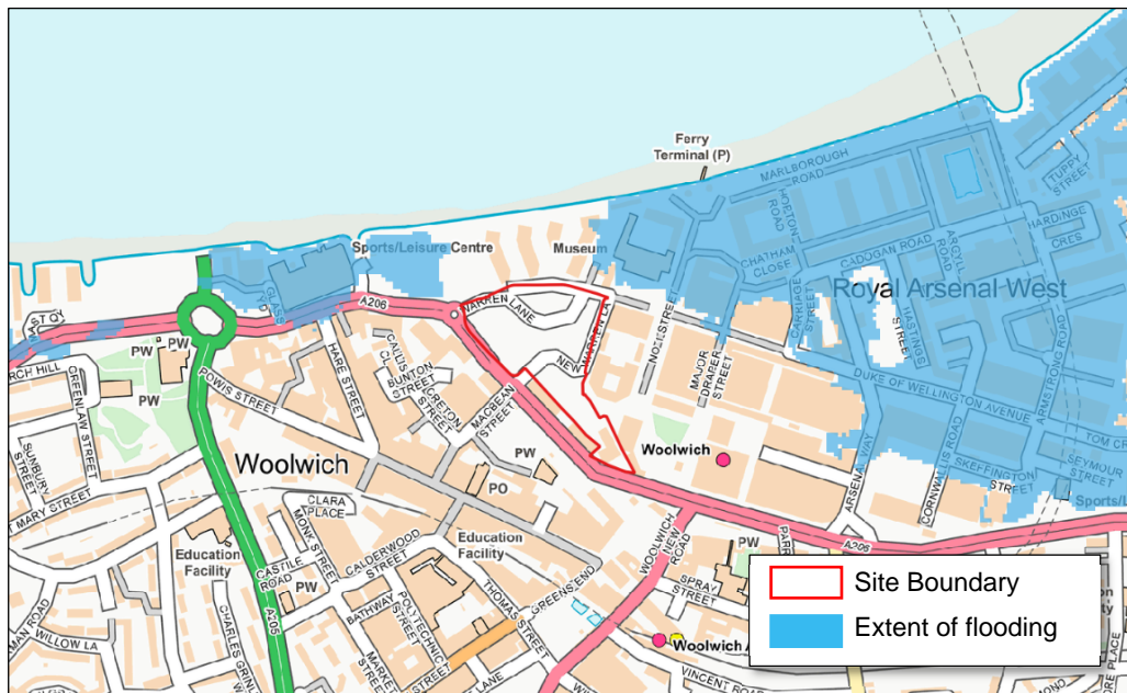
Figure 4.1- Extent of flooding following a breach in the flood defence infrastructure during an extreme event. Model results extracted from the Thames Estuary Breach Assessment (2018) (© Environment Agency 2023).
