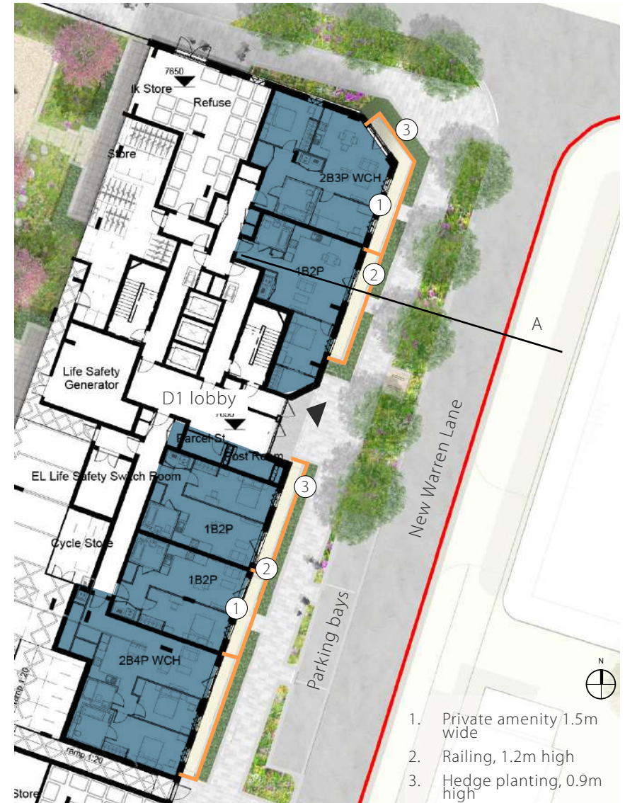
Building D1 Ground floor flats
