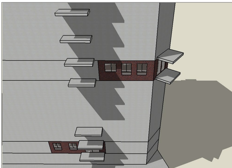
Figure 5: External shading example from DesignBuilder.
