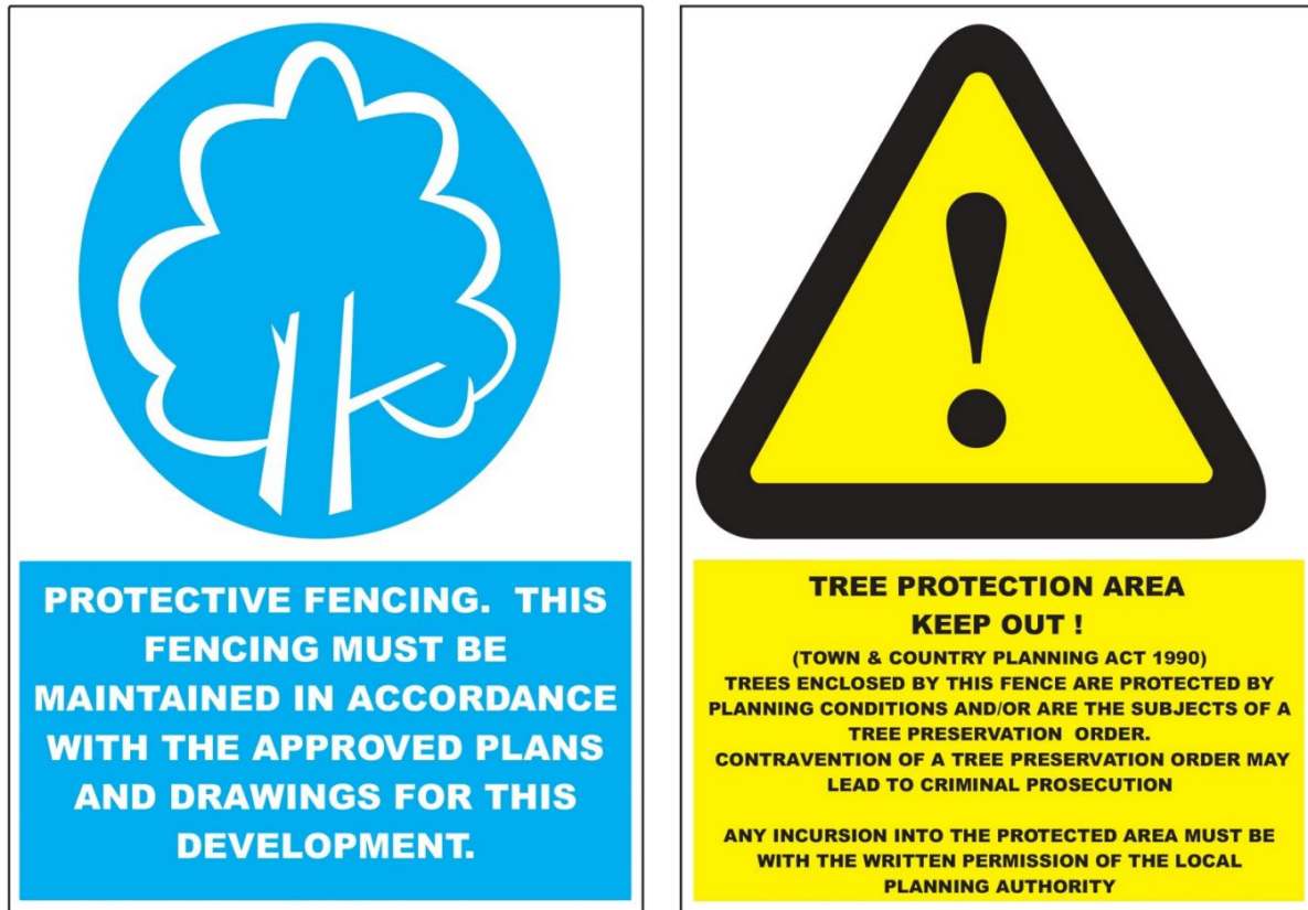
Figure 3. Example of all-weather sign to be attached to protective fencing at 3 metre spacings
