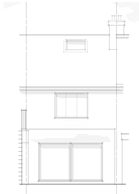
PROPOSED REAR ELEVATION (facing due west) SCALE 1:100
