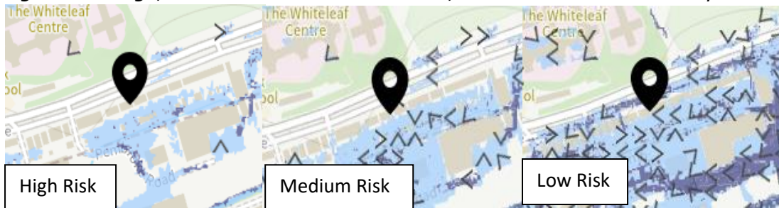
Figure 6b – High, Medium and Low risk scenario; surface water flood risk velocity.
