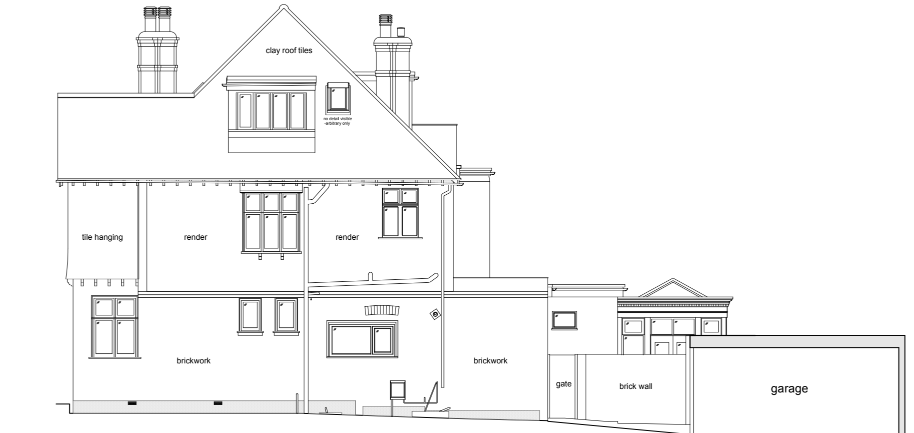
Side Elevation (North) Existing
