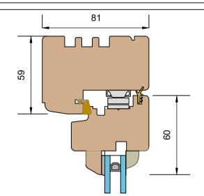
**Timber Casement Window** Head Detail [Scale 1:2]
