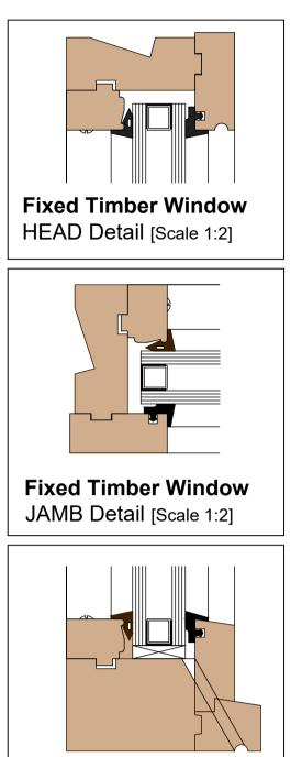
**Fixed Timber Window** CILL Detail [Scale 1:2]
