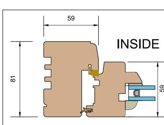
**Timber Casement Window** Jamb Detail [Scale 1:2]
