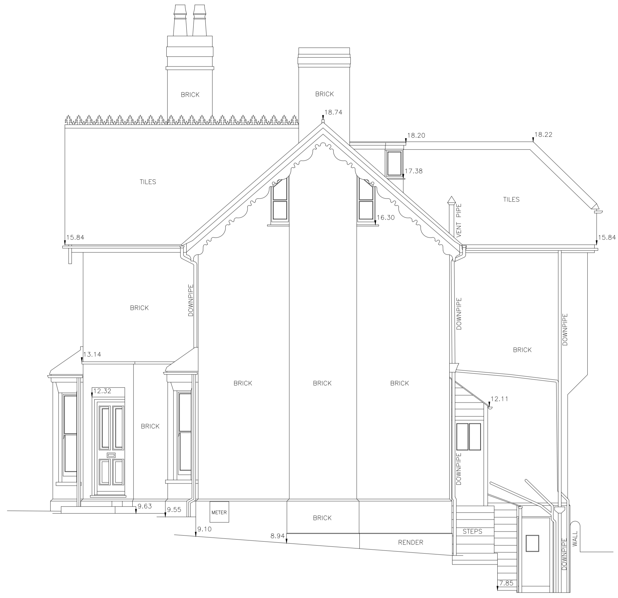
EAST ELEVATION (SIDE)
