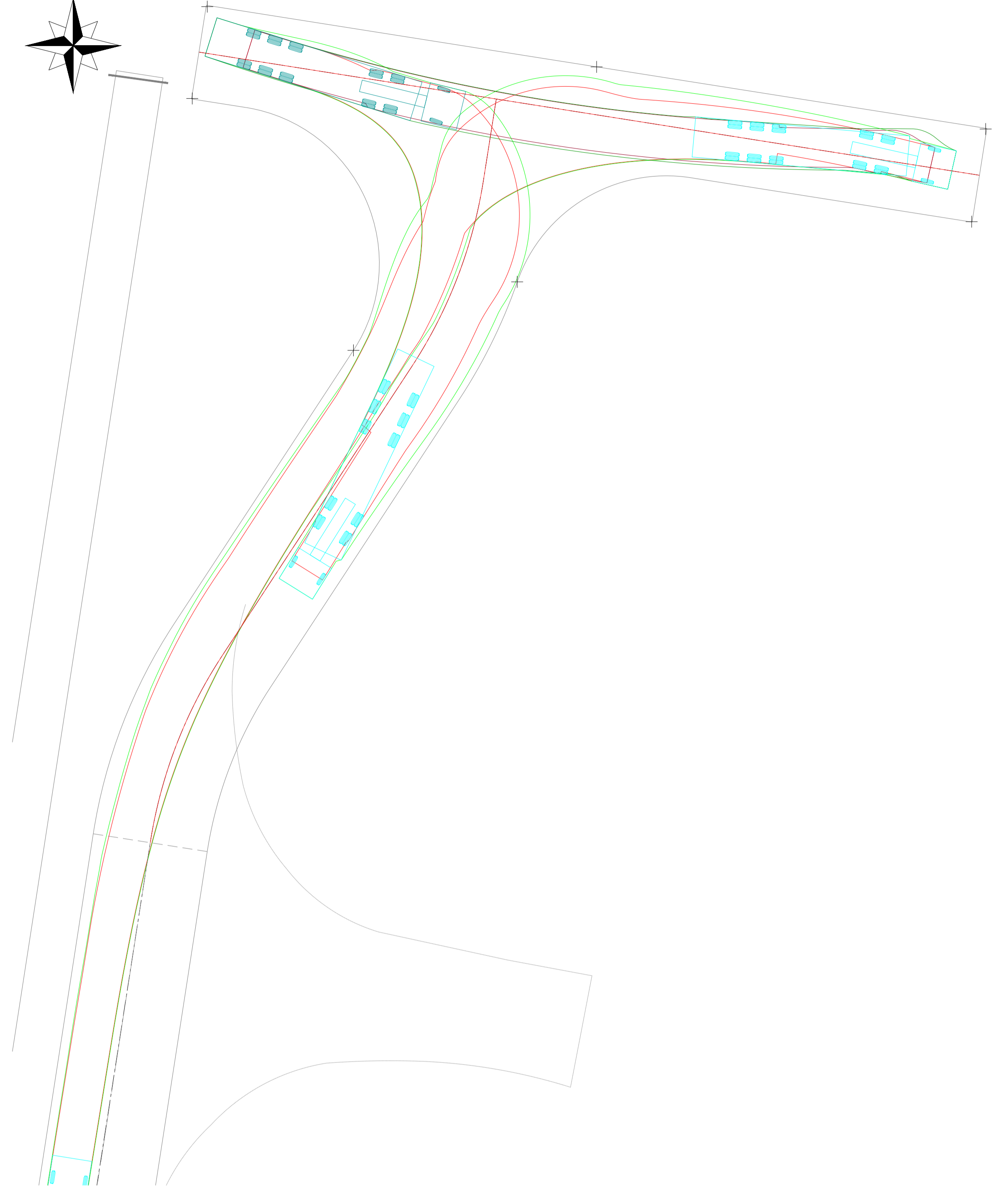
SWEPT PATH ANALYSIS AT TURNING HEAD AT END OF VALLANCE ROAD Scale 1:200
