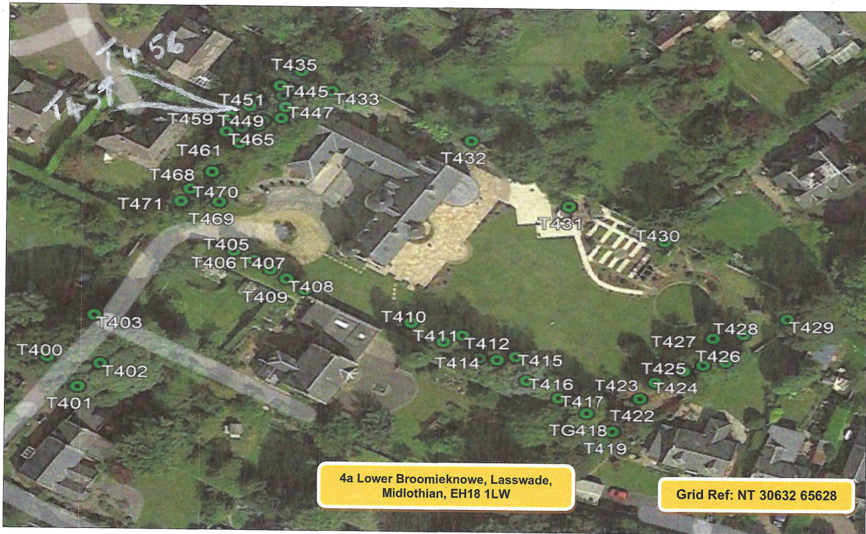
Figure 3: Indicative Aerial photograph showing approximate tree locations and tree tag numbers. Please note that the tree locations were recorded using a Garmin GPSmap 62st, portable GPS unit.
