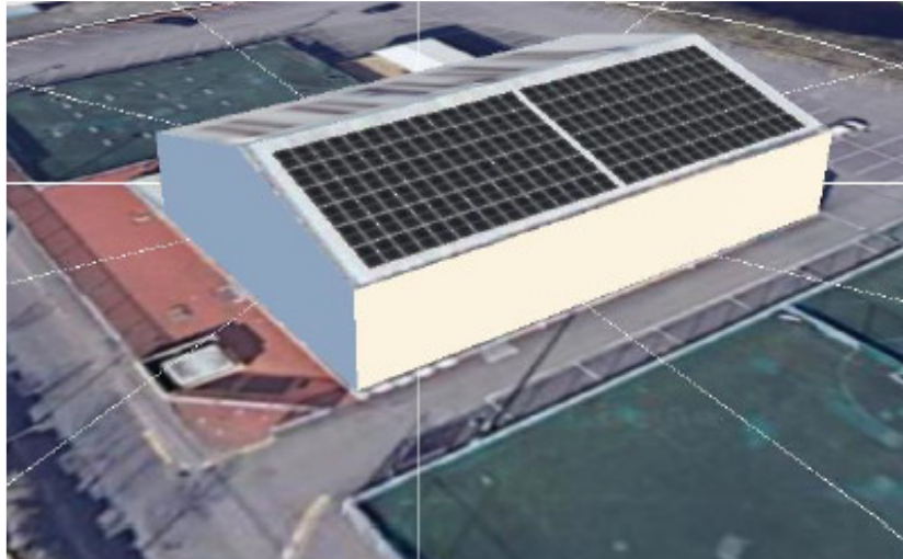
Figure 2: Montage of proposed array arrangement
