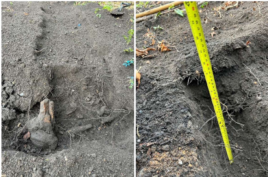
Photo 6 (left); root bole and associated broken root encountered in Area 3. Photo 7 (right); Section of Area 3 excavation, showing excavation depth with small diameter roots present.
