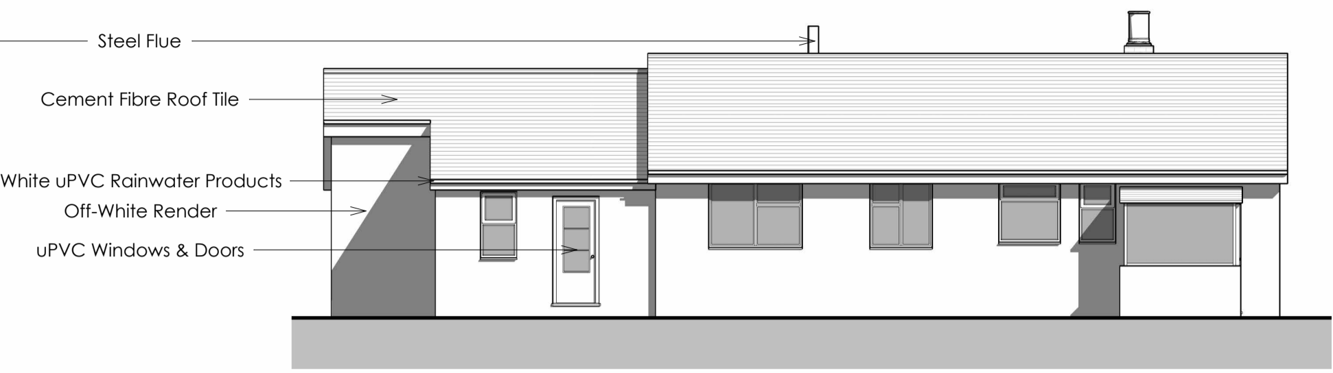
4 Proposed South East Elevation 1 : 100
