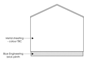
Elevation 01 1:100 Elevation 02 1:100
