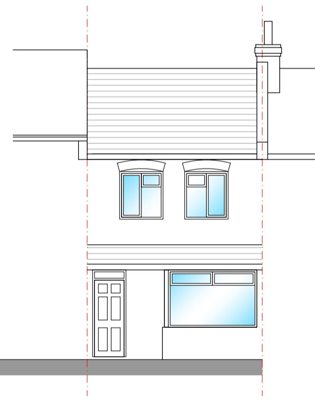
Existing Front Elevation 1:100 @ A1
