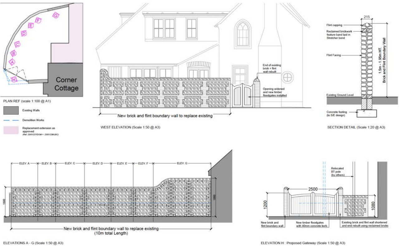
Figure 11: Proposed replacement flint boundary wall and entrance
