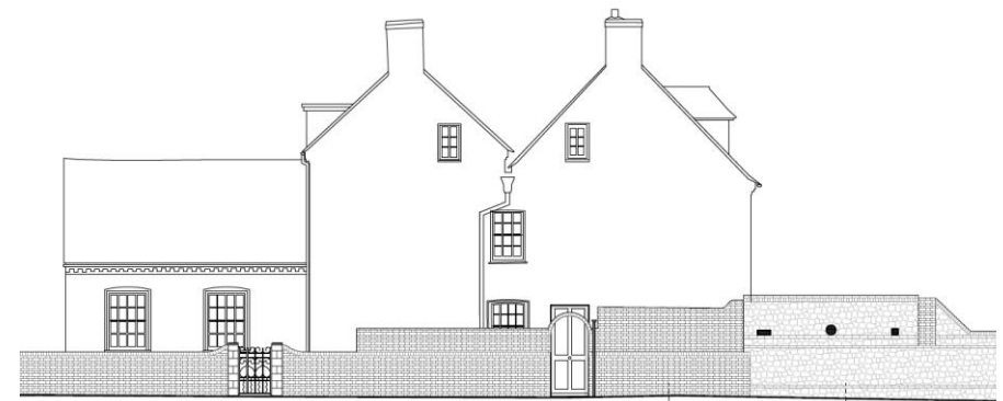
Figure 4. Proposed east elevation showing retention of walling
