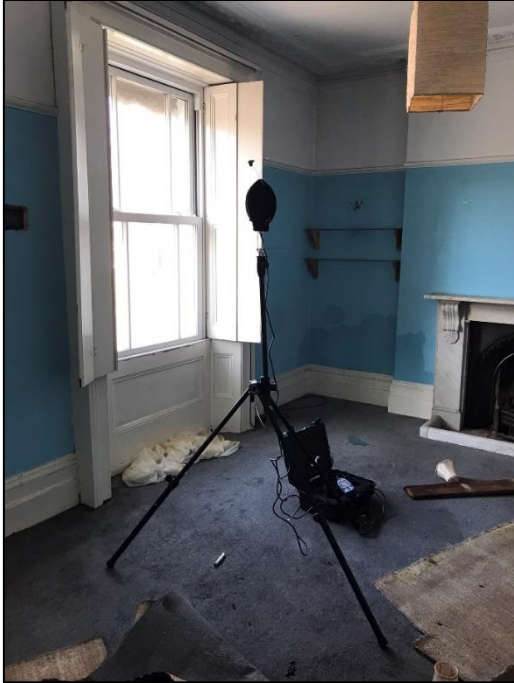
Figure 3 Internal unattended measurement position
