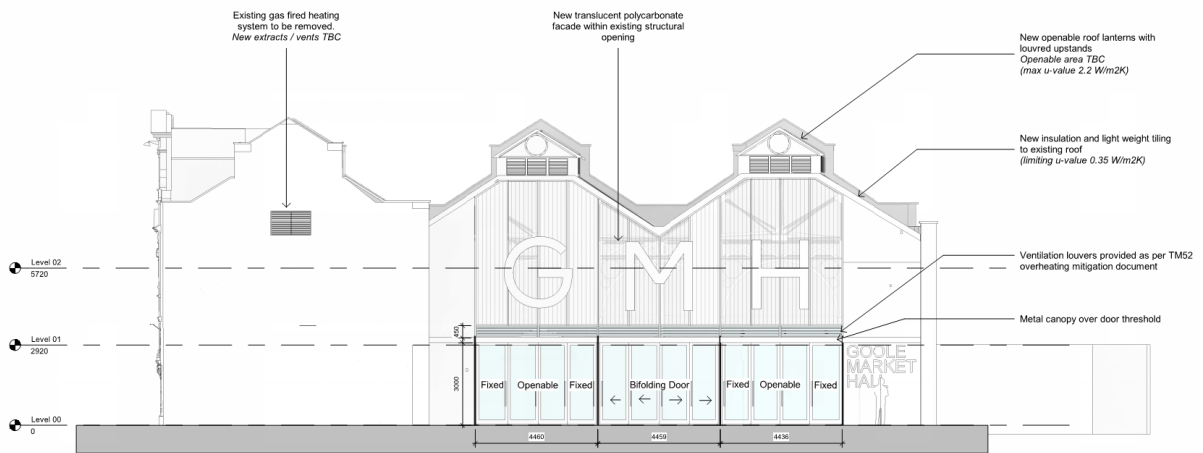
Figure 2 - Drawing showing doors to north facade that are to be opened for large events
