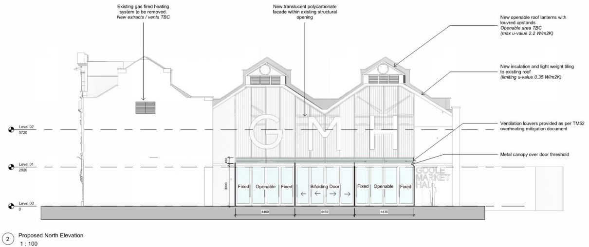
Figure 2 - Drawing showing doors to north facade that are to be opened for large events
