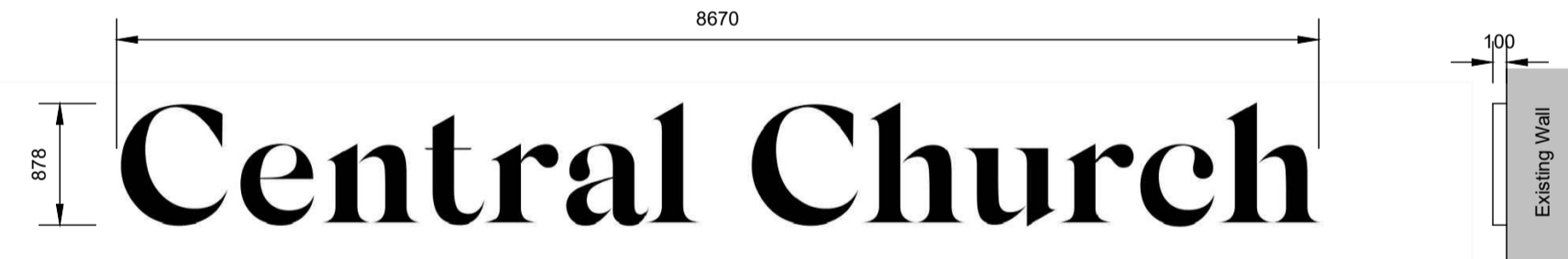
Sign 4 100mm white boxed out lettering. Side of box black Lit with white internal LED lighting Font : Silk Serif bold Scale 1:50
