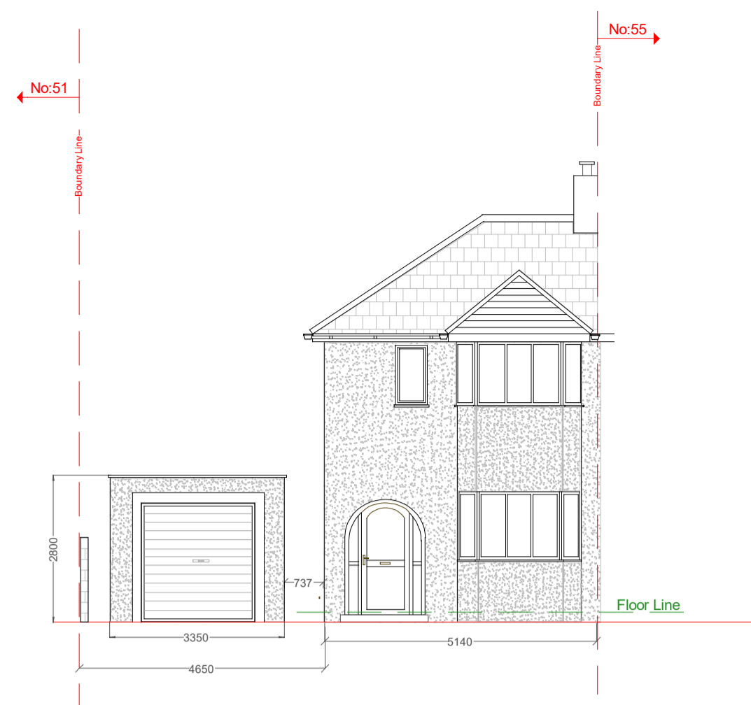
Existing Front Elevation 1:100
