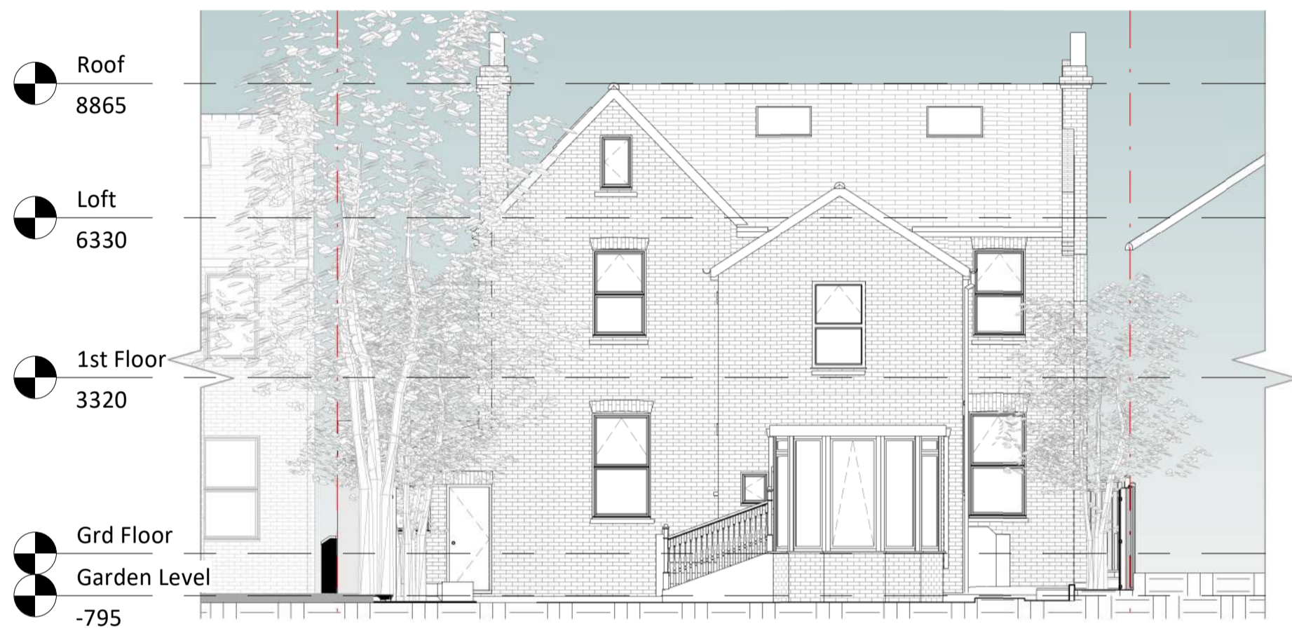
3 Existing Rear Elevation 1 : 100
