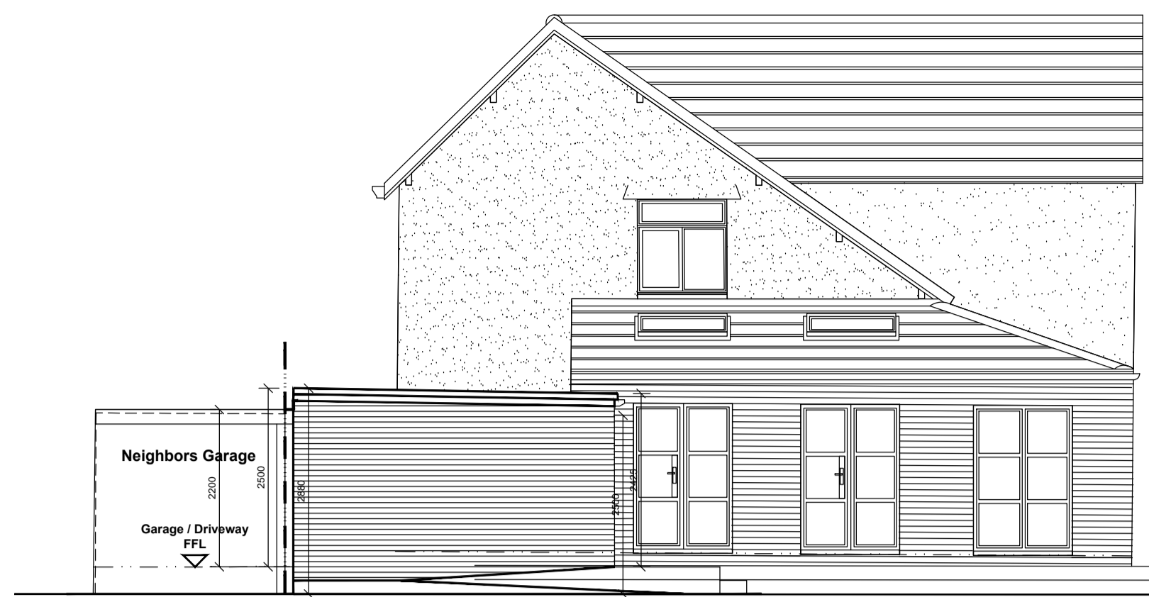
Proposed Rear (NW) Elevation Scale 1:75 @A1
