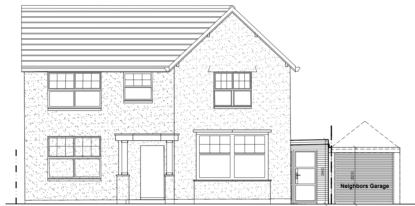
Proposed Front (SE) Elevation Scale 1:75 @A1
