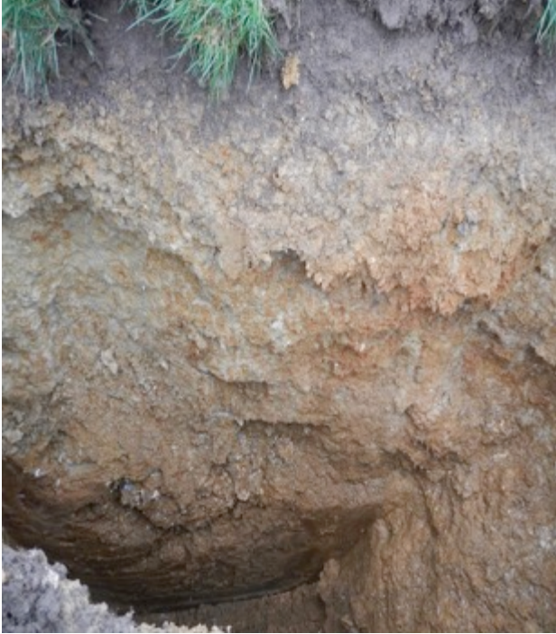
photo to right: flinty pocket giving rise to water ingress
