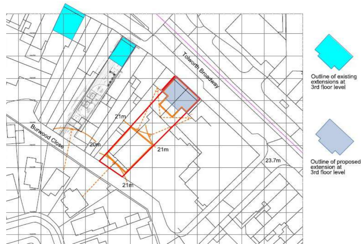
Capacity study/ site setting out with orange line indicating maximum volume of proposed building at 1st and 2nd floor
