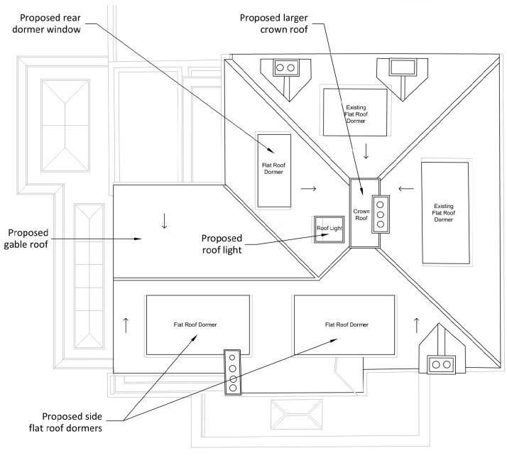
PROPOSED SECOND FLOOR PLAN Scale 1:100 @ A3
