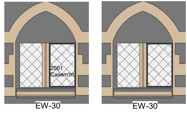
EW-30 Existing - metal windows in timber subframe, leaded glass EW-30 Proposed - refurbish window and leaded lights, replace casement, providing internal secondary glazing to face of window reveal
