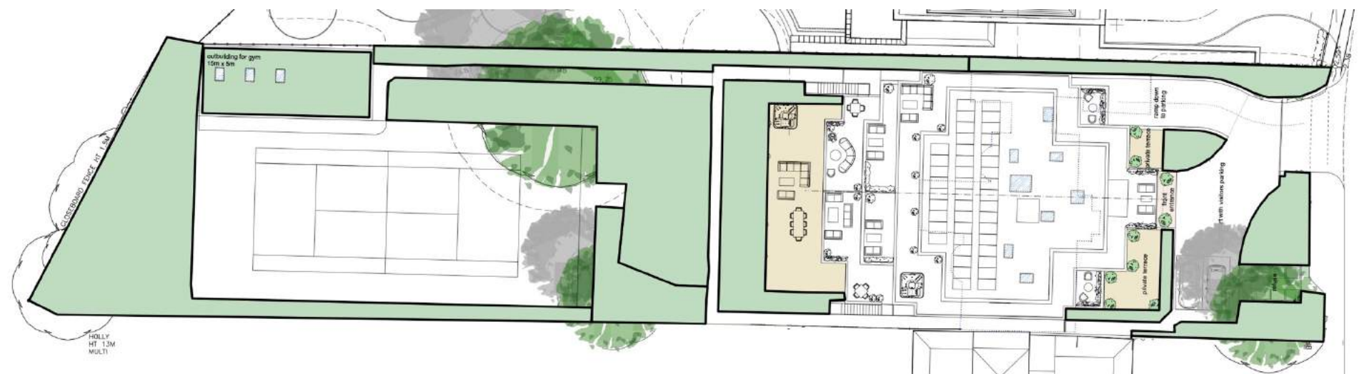
Above: Proposed Site Layout with Soft Landscape Areas highlighted in light green – approx. 990 sq.m
