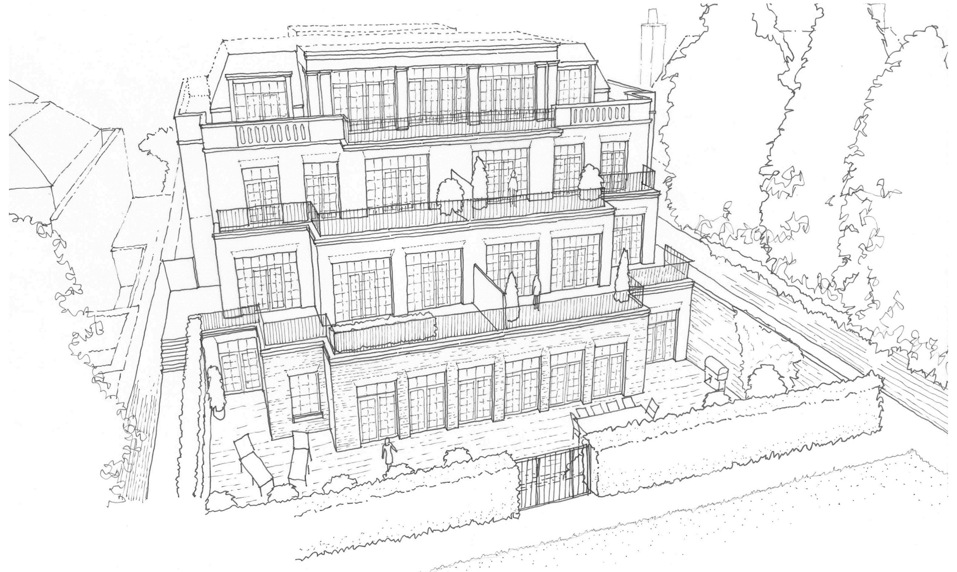
Above: Early Overhead sketch view from the gardens showing larger glazed openings with views over the gardens and large private terraces. Building is also set back at the sides on the garden elevation to reduce impact on neighbouring properties
