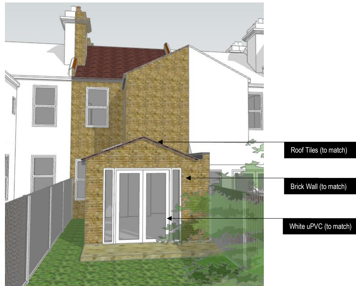
Proposed Ground Floor Rear Extension view
