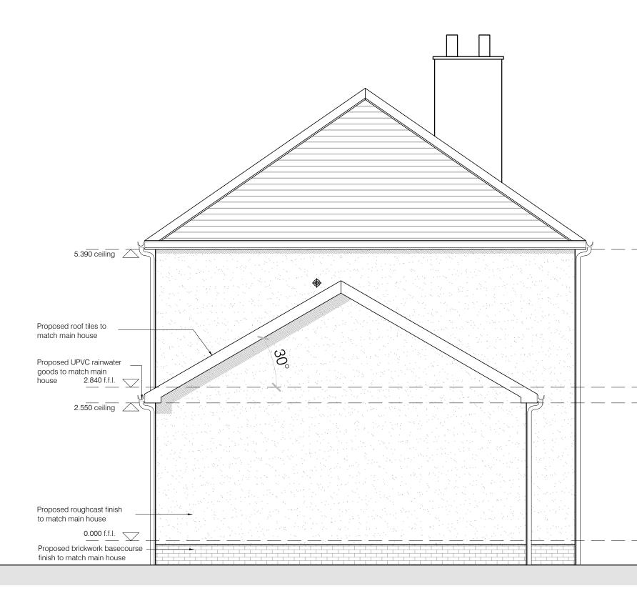
Proposed East Elevation 1:50 @ A3
