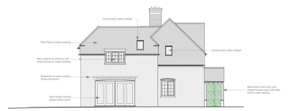
Side Elevation Proposed Scale: 1:100
