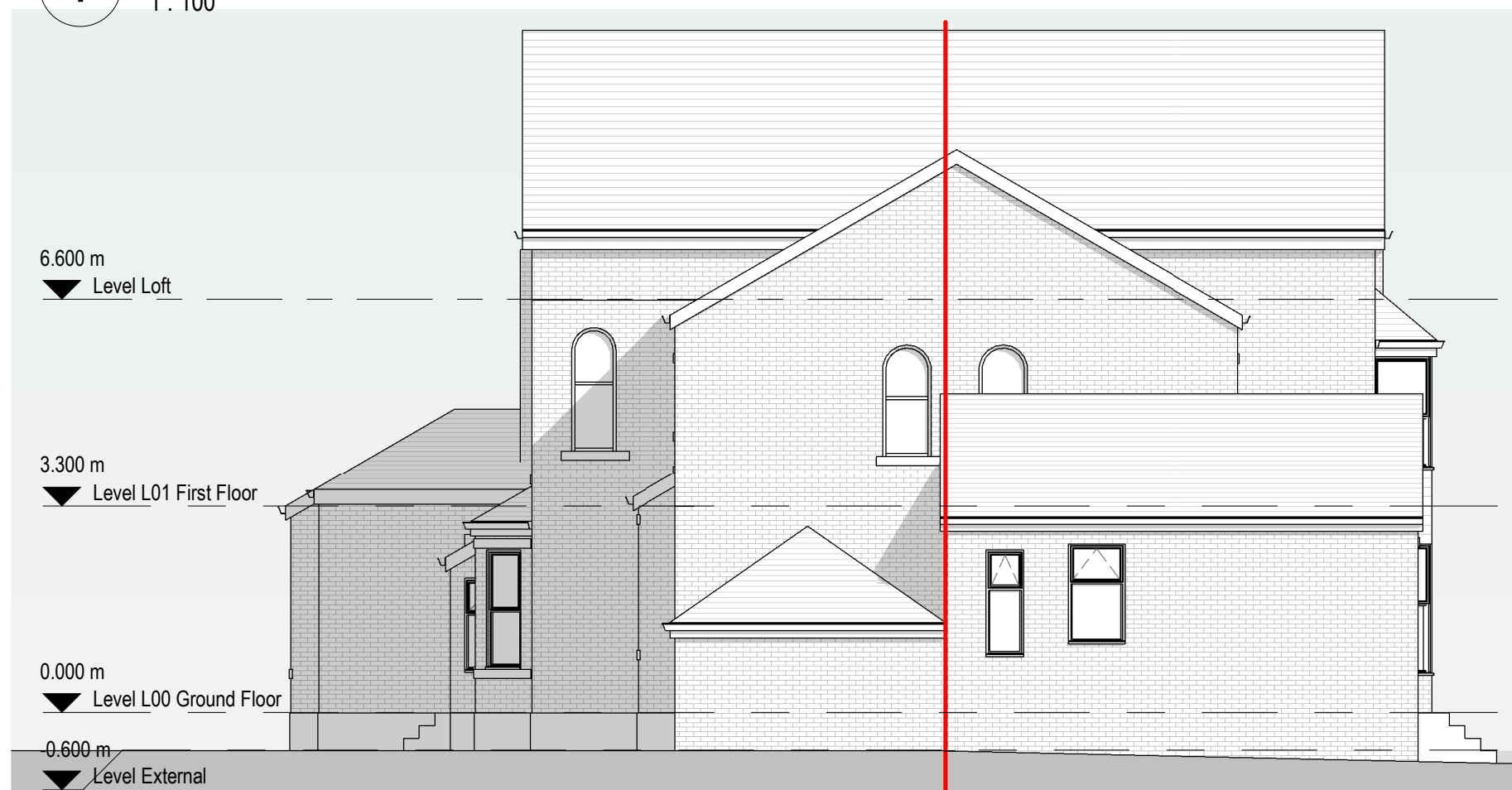
2 Existing West Elevation 1 : 100
