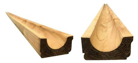
George Hill suggests a life expectancy of 10-15 years for the guttering if the surfaces are treated with an appropriate oil such as shellac. Furthermore, coating with bitumen would hopefully increase its lifespan to a possible 20-25 years. It is supplied with a measurement of 140mm x 75mm with a planed finished size of 63mm x 121mm. The timber guttering will be fixed to the existing gutter gallows with stainless steel screws.
