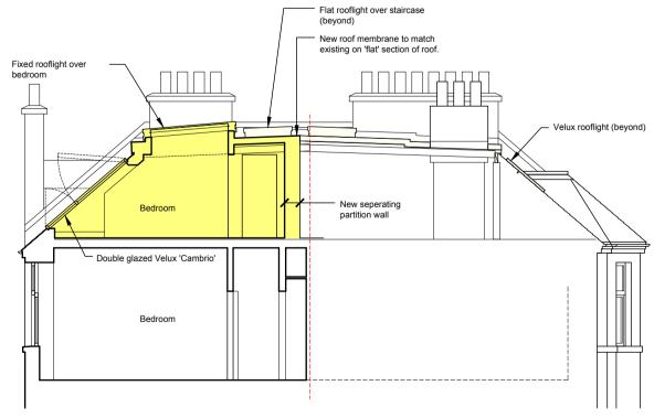
Proposed Section B-B Scale 1:100 @ A1
