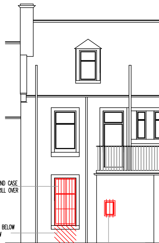
EXISTING REAR ELEVATION REMOVALS SHOWN IN RED
