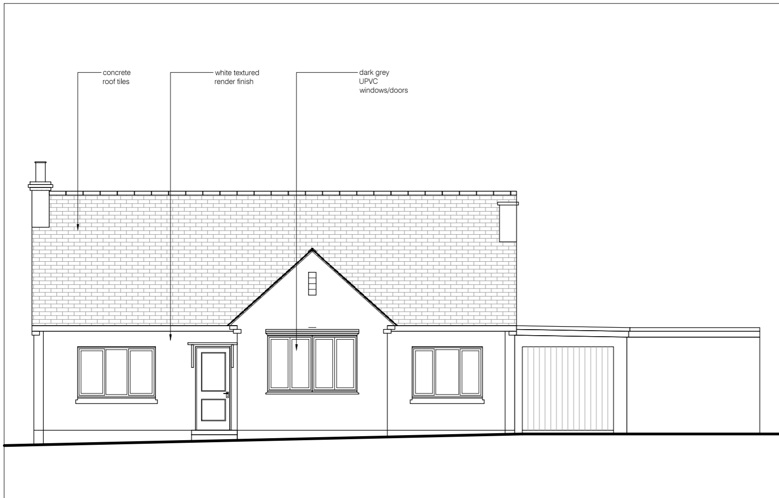
01 EXISTING EAST ELEVATION 1:100
