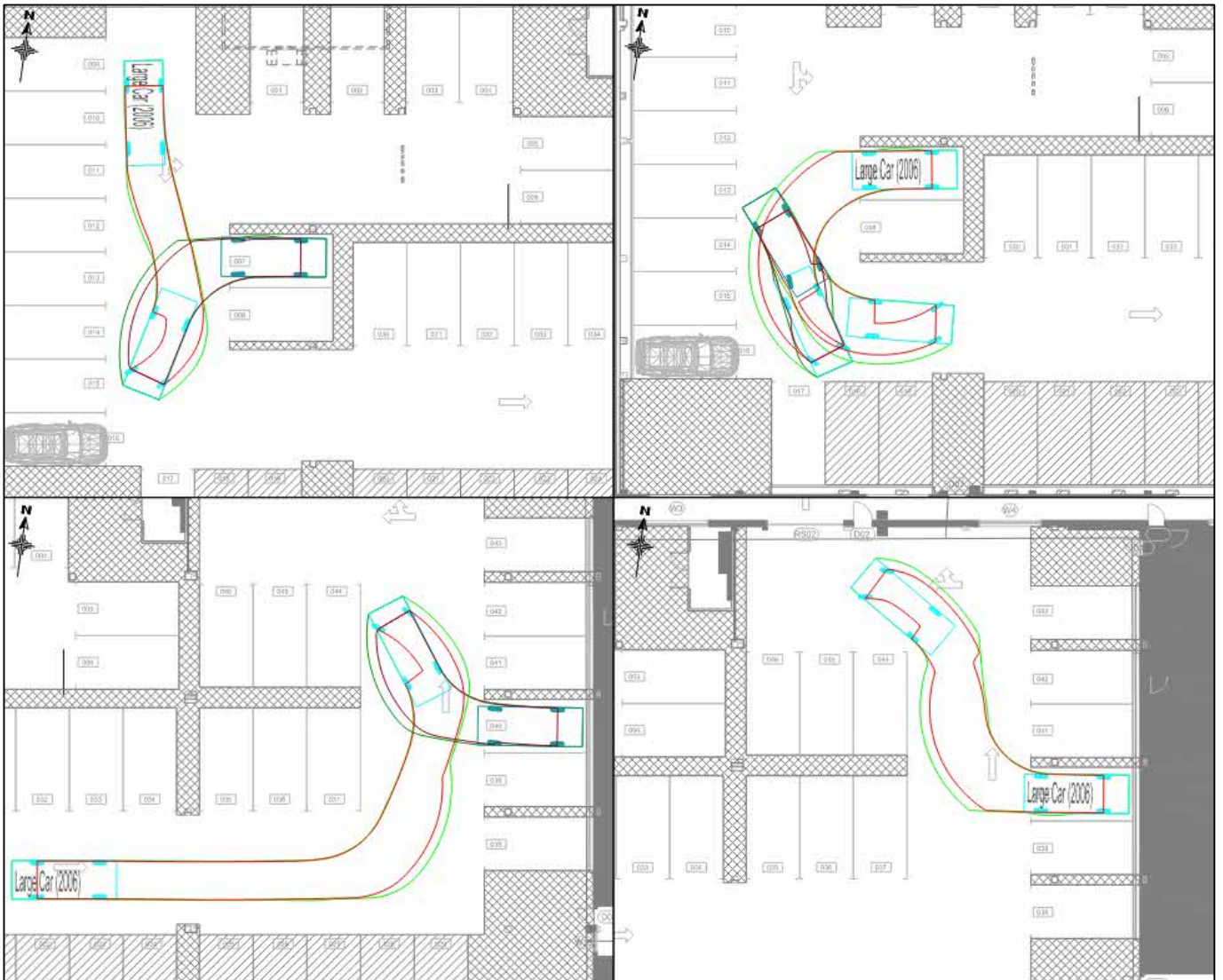
Figure 3-2: A large car entering and exiting the proposed car park and accessing/ egressing from bays
