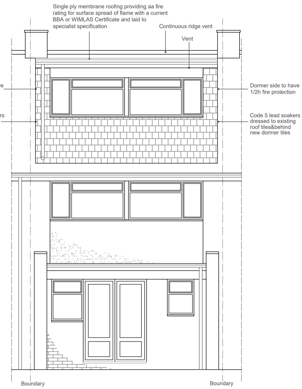
PROPOSED REAR ELEVATION (scale 1:50)
