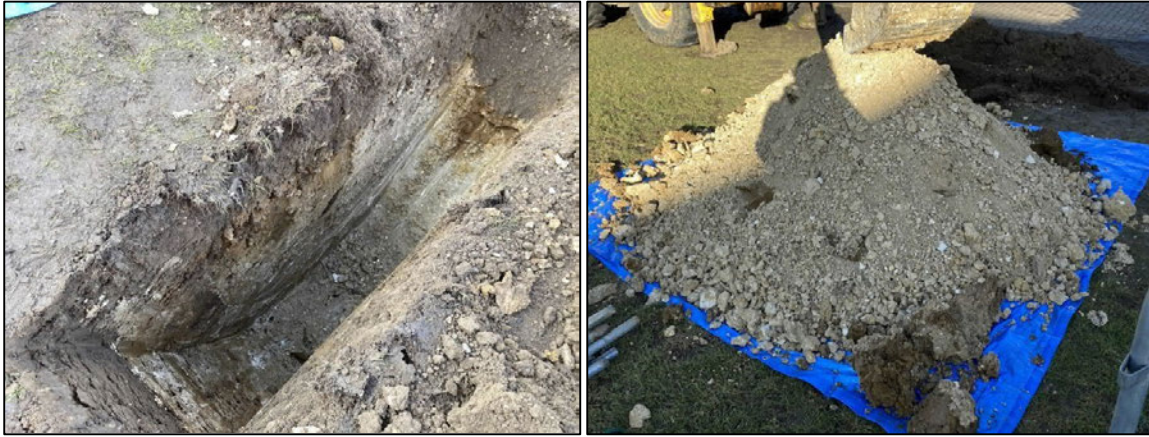
Insert 8 - View of fine-grained Lowestoft Formation in TP102
