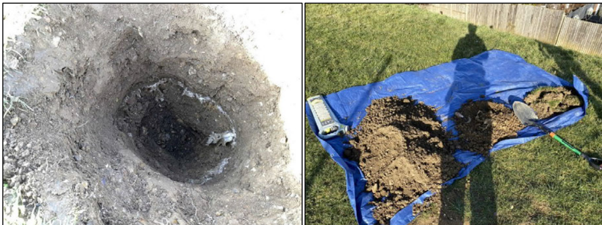
Insert 7 - View of ground conditions and arisings in HPO3. Note the geotextile at around 0.4 m bgl in the left picture.
