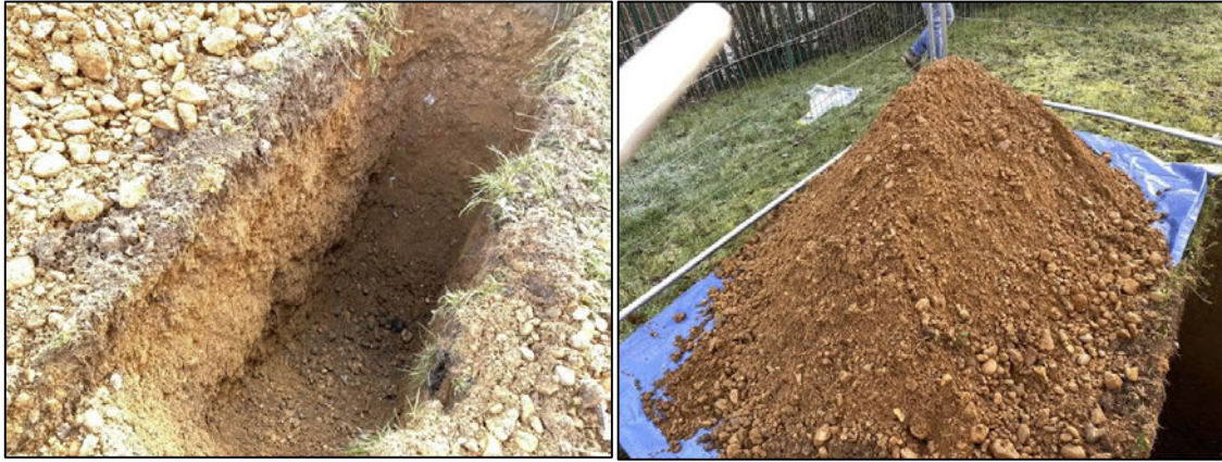
Insert 9 - View of coarse grained Glaciofluvial Deposits in TP104.
