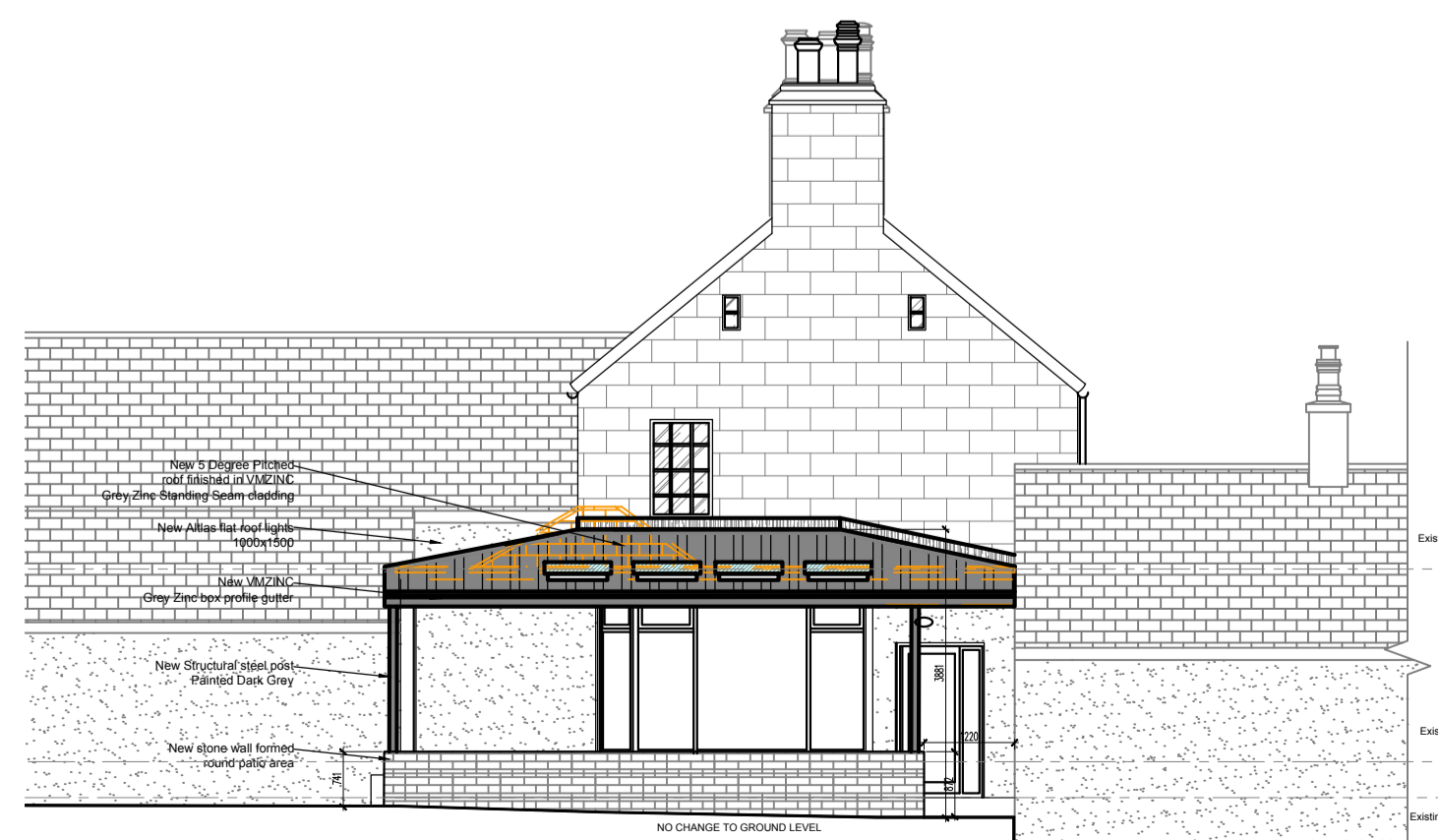
Proposed West Elevation 1:100
