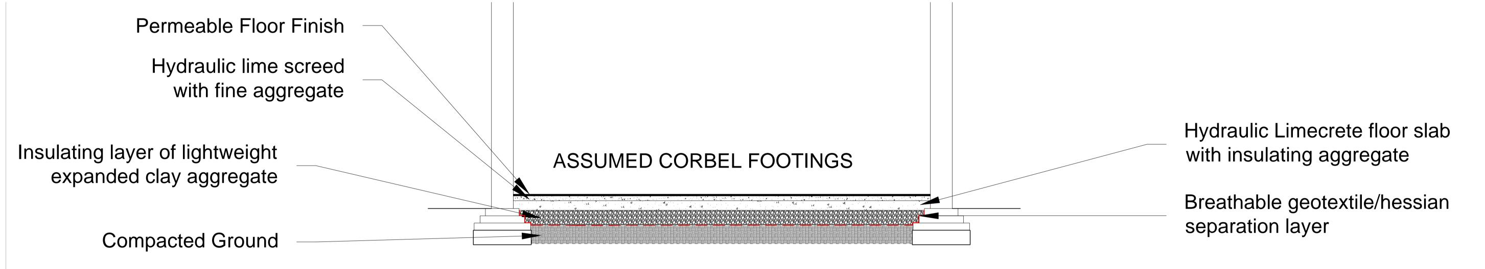
GROUND FLOOR CONSTRUCTION - SECTION OPTION A
