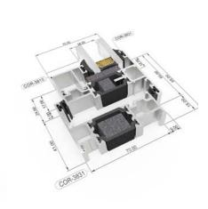
Hinged window system with thermal break and a slim sideline of just 65 mm, which allows a great brightness inside the room. With a modern aesthetic of straight lines, it has profiles tailored for residential and commercial projects, and both for new build and renovation. This system also stands out for its ease in fabrication and assembly, offering excellent performance in thermal and acoustic tests.
