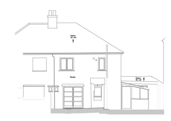
1 ELEVATION Front Elevation SCALE 1: 100 2 ELEVATION
